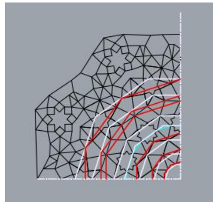
Figure 15: Axes of the geometries of the muqarnas of the Sahip Ata mosque
